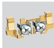
External wiring clamps feature large head brass screws (#10) for superior torque values. Visible brass terminal screws and clamps, with a unique strand containment feature, ensure 100% clamping of wire strands, reducing heat buildup.
