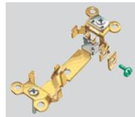
One piece, all brass, mounting strap with integral ground contacts. The safest, most reliable design for a low resistance flow of fault currents. Oversized "bell" shaped ground contacts, along with nickel plated steel retaining shields, help minimize damage to the grounding system during abrupt pullout. Barbed brass locking arms keep the faced locked in place to diminish potential for face/base separation. Back wired ground terminal reduces installation time and increases convenience.
