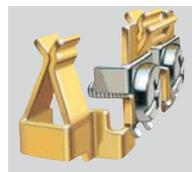
The patented "bypass" contact design incorporates high-conductivity materials with superior spring characteristics for increased contact force and secure connections. Improved contact performance reduces heat buildup and ensures a reliable, uninterrupted flow of power.
