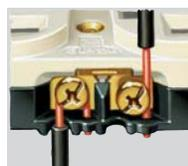
Patented anchor hole and wire restraint feature. Anchor hole helps form solid wire around terminal screw. Wire restraint feature provides strain relief when pushing receptacle into the wall box (HBL5242/HBL5342 series).
