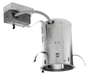
PL513RE TC Fluorescent Remodel Housing TC remodel housing, requires 3" spacing from insulation. 120V thru 277V HPF Electronic Ballast. 13W 4-pin Quad CFL
