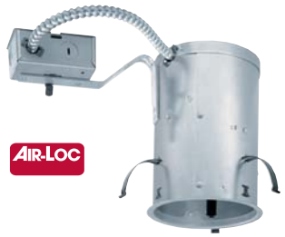
IC20R IC Remodel Housing Energy-efficient, Air-Loc housing can be covered with insulation. Installs from below ceiling. 12½" L x 5⅞" W x 7½" H Ceiling cutout: 5⅞"
