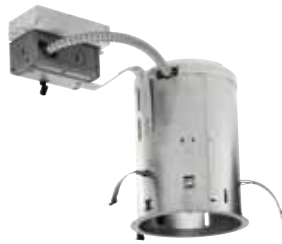
PL518RE TC Fluorescent Remodel Housing TC remodel housing, requires 3" spacing from insulation. 120V thru 277V HPF Electronic Ballast. 12½" L x 5¾" W x 7½" H Ceiling cutout: 5½"
