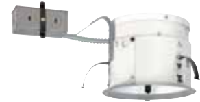
TC2R TC Remodel Construction Requires 3" spacing from insulation. Installs from below ceiling. 13¾" L x 7⅞" W x 7¼" H Ceiling opening: 6⅞"
