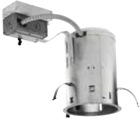
PL526RE Fluorescent Remodel Housing Energy-efficient, CFL housing. 120V thru 277V HPF Electronic Ballast. Requires 3" spacing from insulation. 12½" L x 5¾" W x 7½" H Ceiling cutout: 5½"
