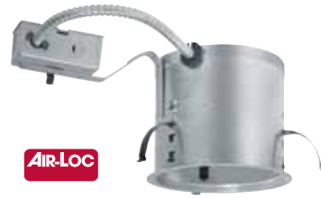
IC21R IC Remodel Housing Energy-efficient, Air-Loc housing can be covered with insulation. Installs from below ceiling. 13¾" L x 7⅞" W x 5¼" H Ceiling cutout: 6¾"
