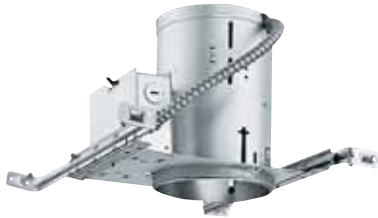
TC20 TC Housing Requires 3" spacing from insulation. 12¼" L x 6⅝" W x 7½" H Ceiling cutout: 5⅝"
