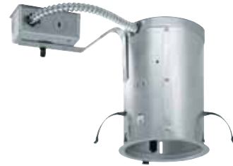
TC20R TC Remodel Housing Requires 3" spacing from insulation. Installs from below ceiling. 12½" L x 5⅝" W x 7½" H Ceiling cutout: 5½"
