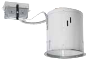
PL618RE TC Fluorescent Remodel Housing 120V thru 277V HPF Electronic Ballast with end-of-lamp-life protection. Requires 3" spacing from insulation. 13¾" L x 7⅝" W x 7½" H Ceiling cutout: 6¾"
