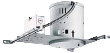
TC2 TC New Construction Requires 3" spacing from insulation. 13" L x 7⅞" W x 7¼" H Ceiling opening: 6⅞"
