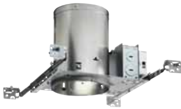
PL518EU TC Fluorescent Housing TC housing, requires 3" spacing from insulation. 120V thru 277V HPF Electronic Ballast. 9¼" L x 6¾" W x 7½" H Ceiling cutout: 5⅝"
