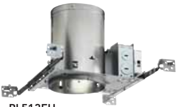
PL513EU TC Fluorescent Housing TC housing requires 3" spacing from insulation. 120V thru 277V HPF Electronic Ballast. 9¼" L x 6¾" W x 7½" H 13W 4-pin Quad CFL
