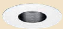
Downlight or Adjustable with Baffle Low Voltage Trim with Transformer 424B-WH Black Baffle 30° vertical adjustment, 358° rotation IC: 35W MR16; TC: 50W MR16 3½" Aperture
