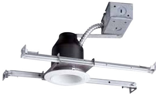
3" Mini-round TC Housing and Trim Shipped complete with trims as listed. Requires 3" spacing from insulation. 6⅞" L x 3⅞" W x 5⅞" H Ceiling cutout: 3¼" sq. TC18-184B-WH Black Baffle TC18-184B-PB Polished Brass TC18-184W-WH White Baffle 60W PAR16 2½" Aperture
