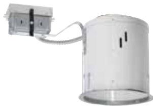
PL613RE TC Fluorescent Remodel Housing TC remodel housing, requires 3" spacing from insulation. 120V thru 277V HPF Electronic Ballast. 13W 4-pin Quad CFL
