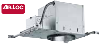
IC2 IC New Construction Energy-efficient, Air-Loc® double wall housing can be covered with insulation. 17¼" L x 9⅝" W x 7½" H Ceiling opening: 6⅞"
