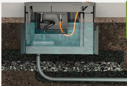
Its NEMA 6P & IP68 Rated "diving bell" design traps and maintains an air pocket, keeping connection points safely away from wet weather.
