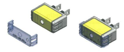
**Step 5.** Apply pressure along the top surface to activate the adhesive and check to be sure the cover clips securely over each end.
