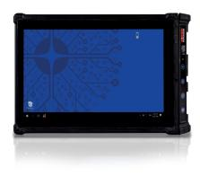
Available in two form factors of 7 inch and 10 inch with a sealed design tested to IP65 and resistant at 1.2 m / 4 ft drop, the TaskBook represents the perfect rugged tablet for indoor warehouses operations.
