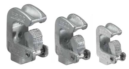
It can't get much easier than the new Kindorf<sup>®</sup> Fast Set Beam Clamp. Simply slide the clamp onto the I-beam flange, and it will remain firmly fixed while you install the threaded rod. When tightened, the threaded rod locks the tongue of the clamp against the I-beam for a fast installation and a superior hold.
