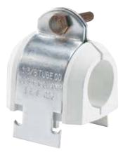
Kindorf® TPE Cable insulator clamps offer a less expensive, lighter weight and non-breakable alternative to porcelain for cable support, and they won't rot like maple clamps. The one-piece thermoplastic elastomer (TPE) insulator is flame-retardant, UV-resistant and chemical-resistant. A tapered flange isolates and protects cable. Available sizes accommodate cables from 3/8" to 41/2" O.D. and fit all Kindorf® channels as well as all 15/8" channel systems.
